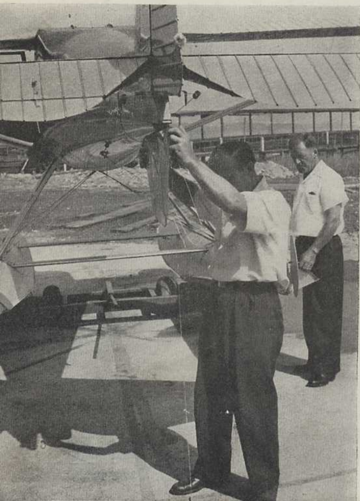
COMPASS CHECK. —Choosing level site and using straight-edge board along which to paint lines, the author trues up straight-edge with astro compass. Using compass rose, ship should be checked in level-flight position (below)
