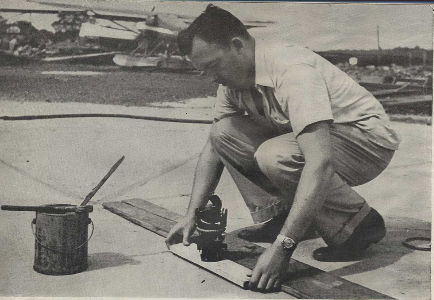
COMPASS CHECK. —Choosing level site and using straight-edge board along which to paint lines, the author trues up straight-edge with astro compass. Using compass rose, ship should be checked in level-flight position (below)
