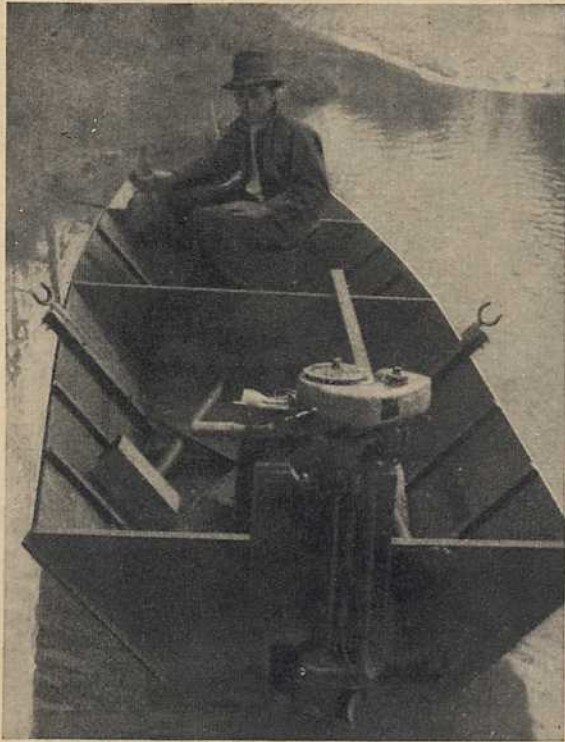
Tunnel stern and flared sides are typical of "Light Dew"—other details are optional. This is a one-piece model
