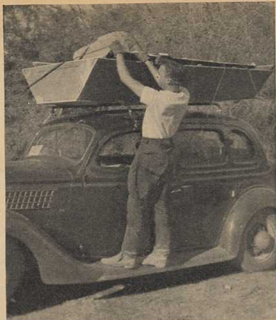
Unbolted and nested, the sectional model makes a remarkably compact load for the car top, lashed to a vacuum-cup carrying frame. If you prefer a trailer, the boat can be built in one piece with heavier planking
